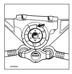
Position the stop ring **(5)**. Tighten the screws moderately.
