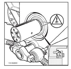
Fit the friction washer (13). Respect the direction of assembly.
