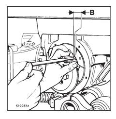
Fit the shim **(6)**. Position the stop ring **(5)**. Respect the orientation. Fit the screws **(4)**. Use a securing product such as "LT 270". Tighten at the recommended torque.
