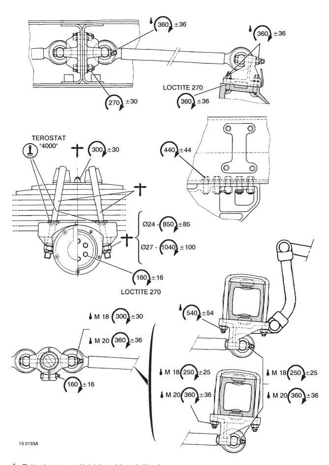
← Tightening torque with lubricated threaded hardware
