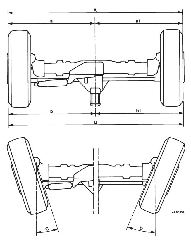
A < B $B=A+2.5\pm1~mm/m$ a < b / a1 < b1 a = a1 $b = a + 1.25 \pm 0.5 \text{ mm/m}$ b = b1 $(C = D) = 13^{\circ}$
